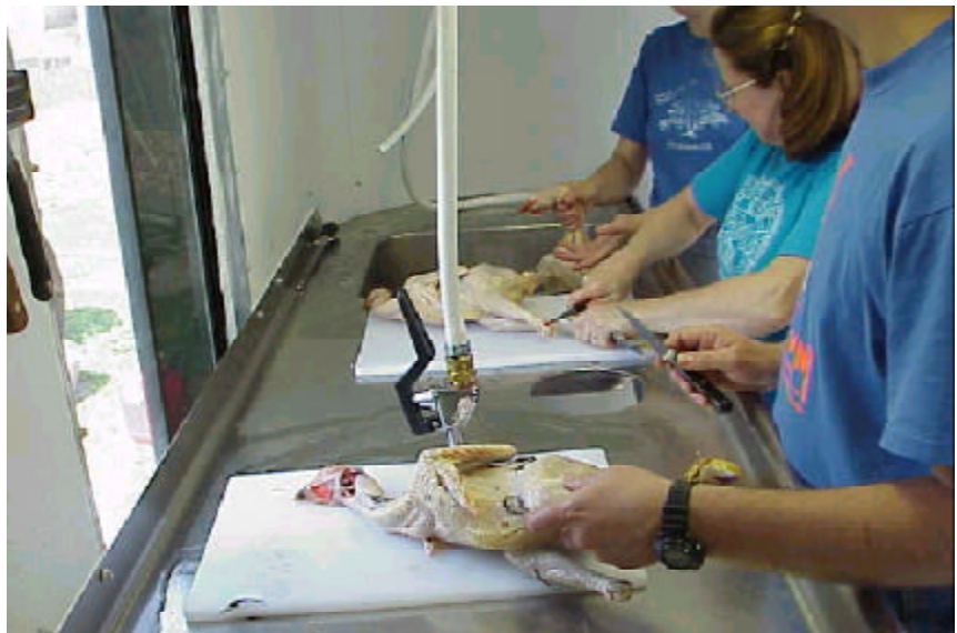
The evisceration area (above) is separated from the scalding and plucking area, which is set off in a screened area. Birds are killed and bled outdoors. Construction materials are easily cleaned, mostly stainless steel.
